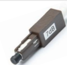
MU/UPC SM Female to Male 1-30dB P/N:GL-FAMUxx
